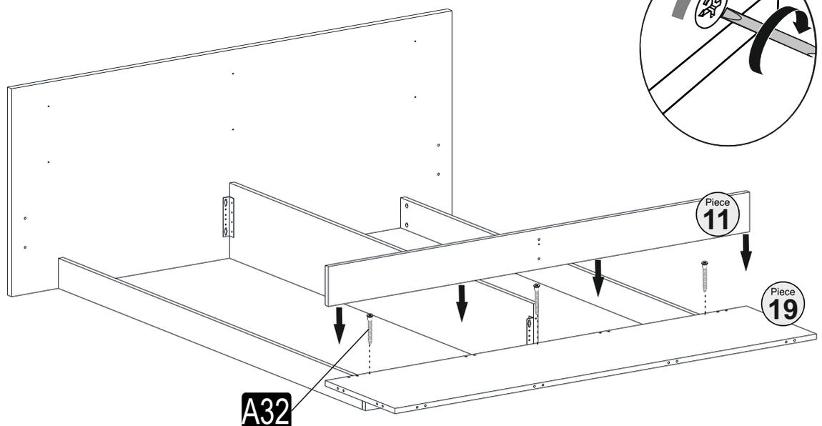
**First of all, fix it to the part no. 19 with screws no. A32. Then fasten piece 11 to piece 19.**
