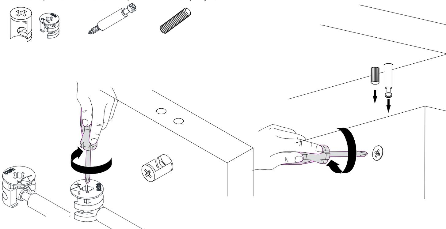
When assembling parts, minifix bodies Place them with their open mouths facing the outside. connected to the minifix shaft Assemble the part it is in so that it coincides with the holes of the other part.
